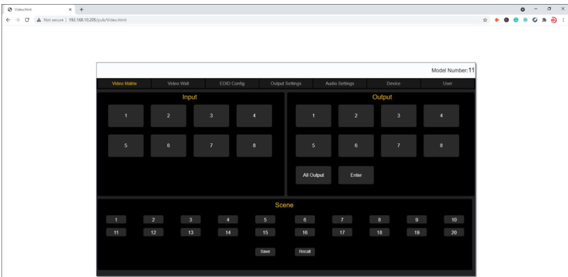
On the input and output buttons, users also can view the active ports by the button color, 3 steps for the switching
