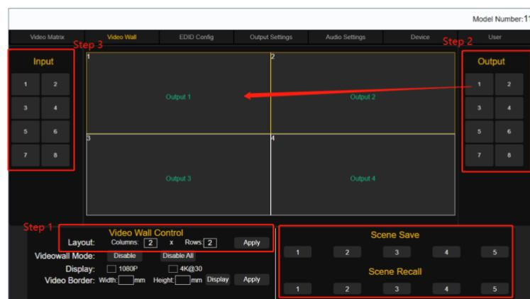
Video Wall box edge in yellow color means that outputs to this VW are all confirmed(use the mouse right click to confirm after drag the outputs)
