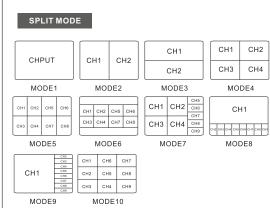
MODE 1: Full screen (IN 1-9 seamless switching mode) MODE 2&MODE 3: Two screen display mode
