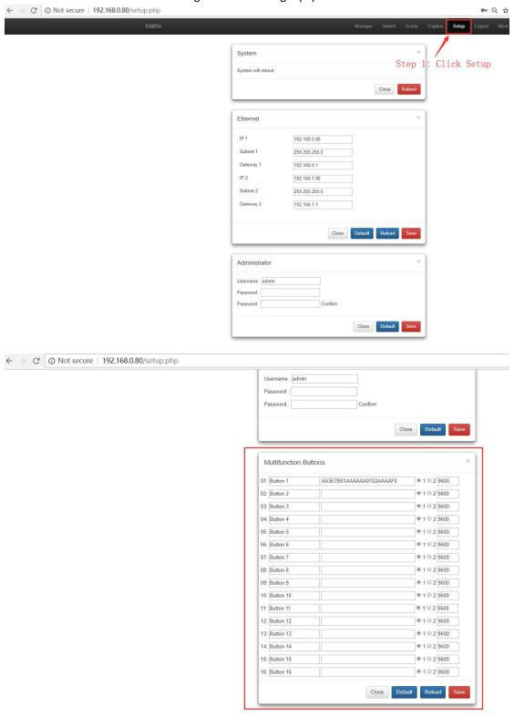
**Multifunction buttons set up**, total we have 16 multifunction buttons at present. We can rename the buttons, Type the HEX code for each button, and baud rate select. Then click "Save".
