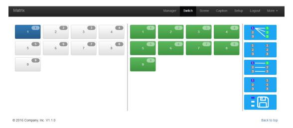
The left side of the long string is input area: Mini99 will have 9 buttons, Mini1818 has 18 buttons, Mini3636 will have 36 buttons. The right side is output area, the buttons are the same with input area. And there're 5 buttons: The 1st for 1 to all, 2nd for 1 off to all, 3rd for 1 to 1, 4th for all off, the last one is for scene save and recall. (Change names can be done in Caption interface)
