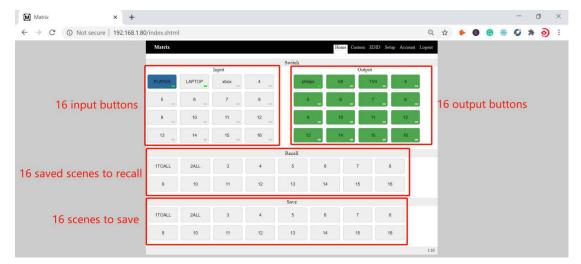
On the input and output buttons, users also can view the active ports by the indicator:
