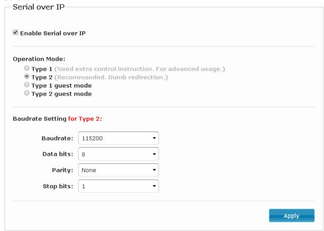
This function setup Serial (RS232) signal sends from network
