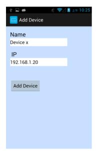
Enter the name of matrix then touch 「Add Device」 to finish setting Notice: Name should be unique, not allow duplicate
