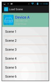
Touch scene column to load saved channels setting for all output It will return to Load Scene page automatically. (Default is Output 1 to Input 1, Output 2 to Input 2 and so on...)
