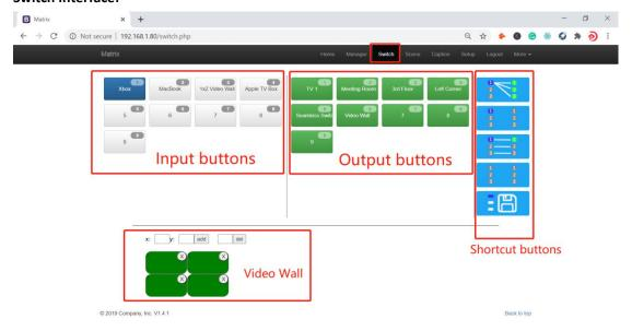
Users can do the input sources switching by clicking the Input buttons first, then pressing the Output buttons.
