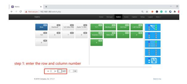
Step 2: Click "add" to create the 2x2 video wall, then drag the outputs to the video wall box.
