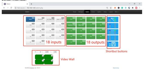
Users can do the input sources switching by clicking the Input buttons first, then pressing the Output buttons.
