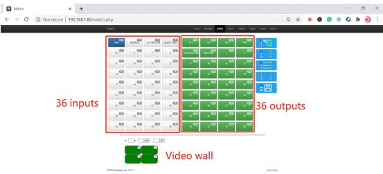
Users can do the input sources switching by clicking the Input buttons first, then pressing the Output buttons.
