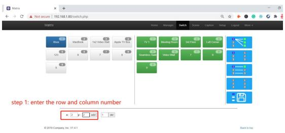
Step 2: Click "add" to create the 2x2 video wall, then drag the outputs to the video wall box.
