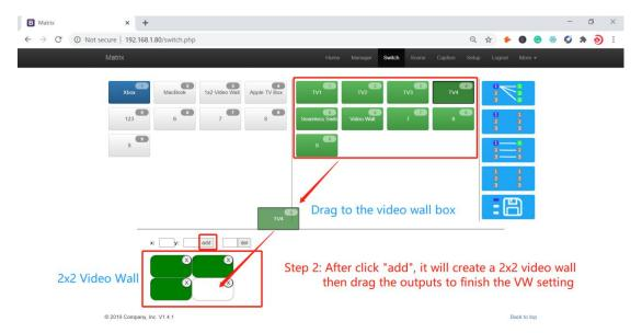
Users can have multiple video walls by the same way to create, for the 9x9 matrix switcher, the video wall configuration will be limited to 9, it means the configuration could be 3x4 video wall.
