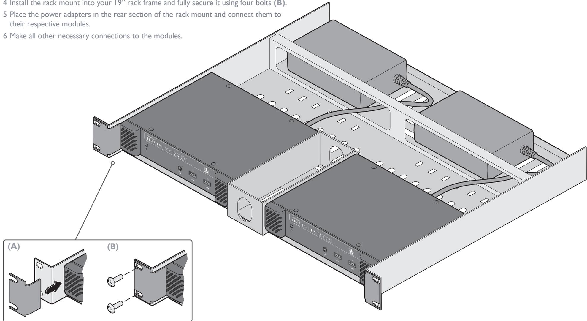
**IMPORTANT:** When mounting the ALIF units (and their power adapters), ensure that the vents are not obscured and that there is sufficient airflow. The operating temperature range is 0 to 40°C (0 to 104°F) and must not be exceeded.
