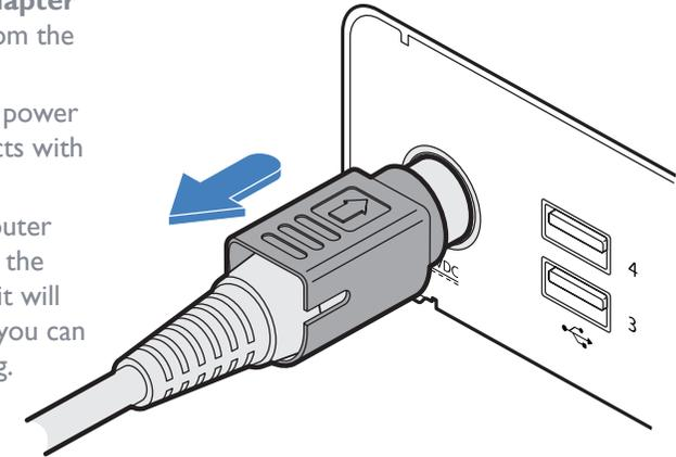
Gently pull back the plug outer body to release the lock
