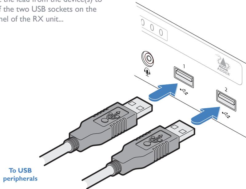
...and/or either of the two USB sockets on the rear panel.
