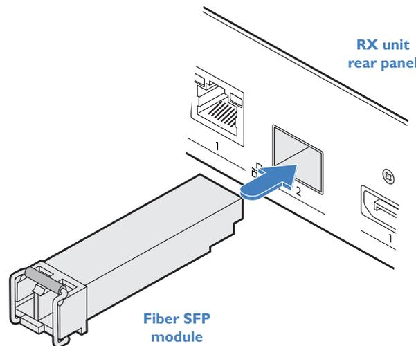
2 Make your fiber connection(s) between the SFP module and either the other ALIF2100 unit or a suitable fiber network switch.
