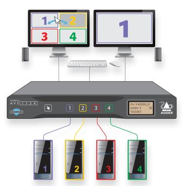
Switching between computers can also be controlled from the smart front panel or by using keyboard shortcuts. Multiple techniques are employed to ensure that no crosstalk can occur between the connected computer channels.
