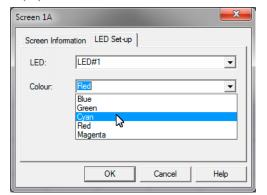
Note: Each LED indicator can only have one colour, so if you associate an indicator with more than one screen and then change the colour on a later screen assignment, it will be changed for all the screens in the list for that LED indicator.
