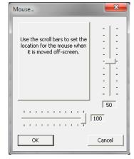
Mouse parking allows you to optionally determine where the mouse pointer for each system should be placed when the focus moves to a different system/video screen. The **Configure** > **Mouse parking...** option displays vertical and horizontal scroll bars. Use the scroll bars to pinpoint the position that should be used to park the dormant mouse on each screen.
