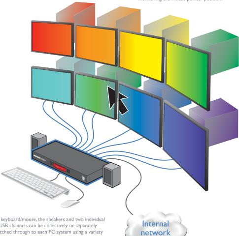
The keyboard/mouse, the speakers and two individual USB channels can be collectively or separately switched through to each PC system using a variety of manual and/or automatic switching methods.
