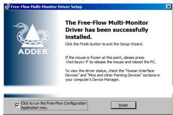
Note: On each PC that you installed the driver, a process called mumoapp.exe will remain running.
