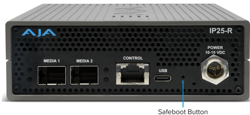
Figure 5. IP25-R (Front View) Safeboot Button
