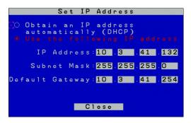
**Note:** 1. If you choose *Obtain IP address automatically (DHCP)*, when the switch starts up it waits to get its IP address from the DHCP server. If
