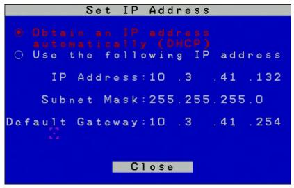
The CN8000A can have its IPv4 address assigned dynamically (DHCP), or it can be given a fixed IP address.
