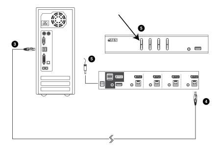
4. At the other end of the USB cable, connect the USB Type B connector to the Type B USB port in the Port 1 KVM section.
