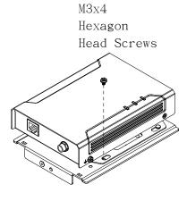
Step B: Screw device to mounting plate.
