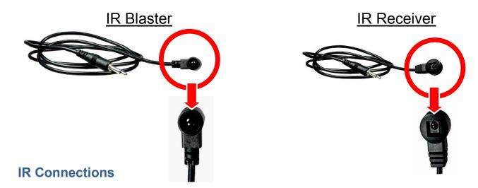
The DXE-CAT Series has the ability to auto detect on the IR port if a receiver or a blaster / emitter is connected.
