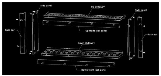
After assembled completely, it will look like below, please note that the Tx/Rx will be installed from the front panel on the installation cage and then locked by the up&down lock panels.
