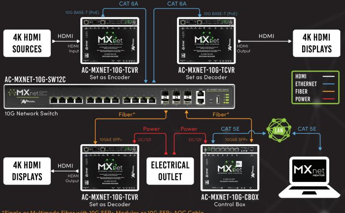
\*Single or Multimode Fiber with 10G SFP+ Modules or 10G SFP+ AOC Cable
