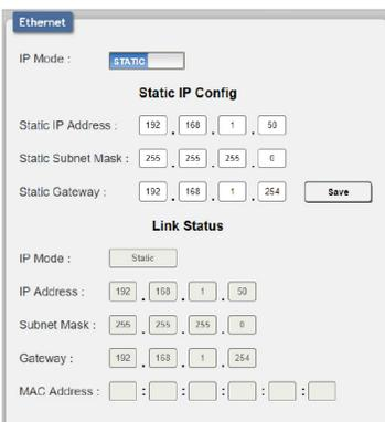
This tab provides controls to change the network settings for the unit. You can manually set the IP address, netmask and gateway address in "Static IP" mode, or you can obtain an IP address automatically by enabling DHCP.
