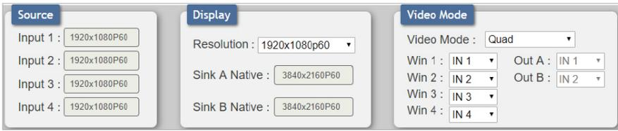
This upper section of the web interface is visible on every tab and provides control over the unit’s operational mode, source selection, and output resolution as well as containing basic information about the currently connected source and display devices.
