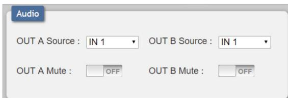
This tab provides control over the audio output behavior of the unit, including routing selection and muting.
