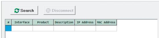
5. After launching the software, power the unit on and then connect it to the PC/laptop using a USB cable. Click on the “
