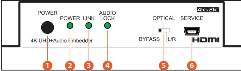
**1 POWER:** Press this button to power the unit on or off.
