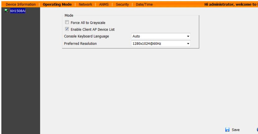
The Operating Mode page is used to set working parameters, as described below:
