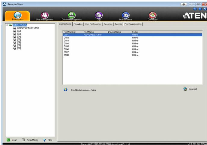
The Connections page is organized into several main areas. All the devices and ports that a user is permitted to access are listed in the Sidebar at the left of the page. After selecting a device or port in the Sidebar, clicking entries on the menu bar (Browser GUI) or tab bar (AP GUI) opens information and configuration pages related to the item selected in the Sidebar.
