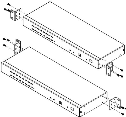
3. Slide the unit into the front or rear of the rack and secure it to the rack.
