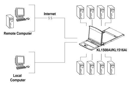
By daisy chaining up to 15 additional switches, as many as 256 computers can be controlled from the original KVM console. An auto-sensing function recognizes the position of each station on the chain, eliminating the need to manually set the position, and a two digit seven-segment LED display on the keyboard module showing each station's position for easy identification.
