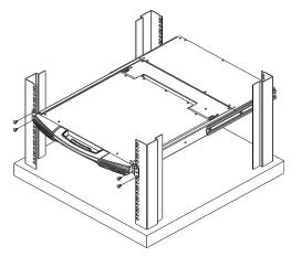
2. While the first person still holds the switch in place, the second person slides the L brackets into the switch's side mounting brackets, from the rear until the bracket flanges contact the rack, then screws the L brackets to the rack.
