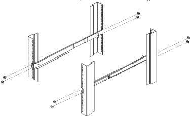
3. Slide the switch onto the support flanges. Use the screws supplied with this package to loosely attach the front of the switch to the front of the rack (only tighten the screws part way).
