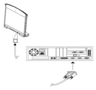
**Note:** On a daisy chained installation, connect the cable to the first station (master) unit. The chained stations (slaves) that are the same model will receive the upgrade via the daisy chain cables.
