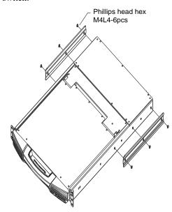
2. Attach the left and right *easy-installation* mounting rails to the inside of the rack. The flange that supports the switch will be to the inside.
