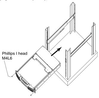
4. Slide the rear attachment sliding brackets along the slide bars until they contact the rear of the switch, then use the screws supplied with this package to attach the bars to the rear of the switch (tighten the screws all the way).
