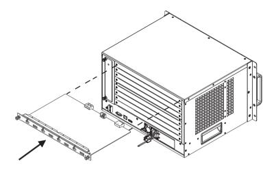
3. Slide an output board into a bottom slot and tighten the screws to secure the board to the VM1600A.
