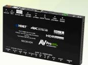
The AC-CXWP-KVM-KIT is a 4K60 4:4:4 18Gbps supported HDBaseT wall plate extender kit over single CAT UTP/STP. This device can take in any HDMI signal and transfer it long distances; simultaneously, it's able to send a USB 2.0 signal (bi-directionally) through the same cable. This makes for the ideal solution for classrooms and conference rooms to work with modern laptops and desktop computers.
