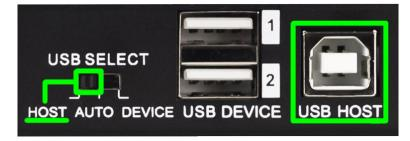
Select DEVICE if you are plugging into the USB DEVICE port (Type A)
