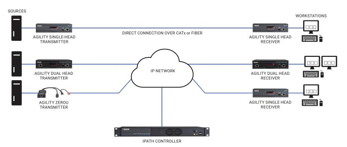
Agility point-to-point and matrix switching setup that connects multiple source PCs and user workstations.
