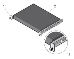
FIGURE 5-5. SWITCH RAILS ATTACHMENT
