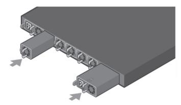
FIGURE 7-2. PSU AND FAN INSTALLATION
