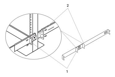
FIGURE 5-3. TWO-POST CENTER-MOUNT CONFIGURATION
