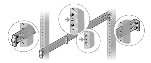
FIGURE 5-1. 1U TOOL-LESS CONFIGURATION
