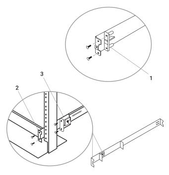
FIGURE 5-2. TWO-POST FLUSH-MOUNT CONFIGURATION
