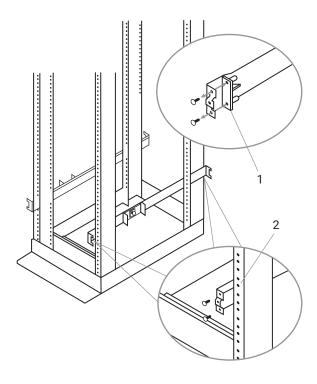
FIGURE 5-4. FOUR-POST THREADED CONFIGURATION
