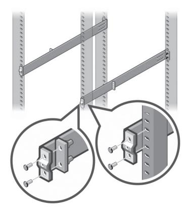
FIGURE 4-5. FOUR-POST THREADED CONFIGURATION
