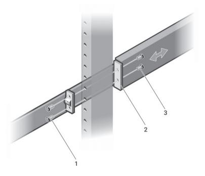
FIGURE 4-4. TWO-POST CENTER-MOUNT CONFIGURATION
