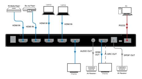
**Note:** Slide the DIP switch to De-embedded mode, the SPDIF Out of Output2 will output the digital de-embedded audio from HDMI Out2.
