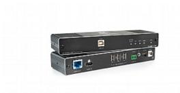
TP-590T is a high-performance, long-reach HDBaseT 2.0 transmitter for 4K60Hz (4:2:0) HDMI, USB, RS-232, and IR signals over twisted pair. TP-590T converts all input signals into the transmitted HDBaseT 2.0 signal. It extends video signals to up 40m (130ft) over CAT copper cables at up to 4K@60Hz (4:2:0) 24bpp video resolution and provides even further reach for lower HD video resolutions
