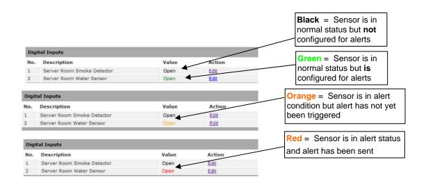
Figure 18-Sensor Values in color have meaning
