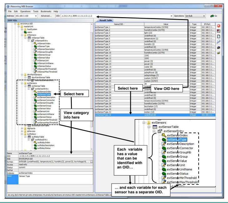
Each RJ45 Sensor port has two OIDs assigned, because the sensors that connect to these ports often have two possible functions (Temperature/Humidity, ACLM-V with two connections, etc.). The image above shows they are numbered sequentially (The "extSensor Type" variable for Port 1 is extSensorType.1 and extSensorType.2, port 2 is extSensorType.3 and extSensorType.4, and so on, for a total of 4 extSensors (RJ45 Sensor) for an E-1W.)
