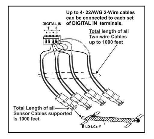
After installation of rope style leak detection sensor in its desired location, **it is very important** to test the sensor to verify correct installation. This applies to **all** rope-style leak detection sensors.
