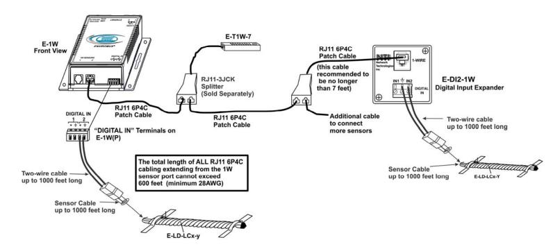
Figure 8- Digital Inputs connected using E-DI2-1
