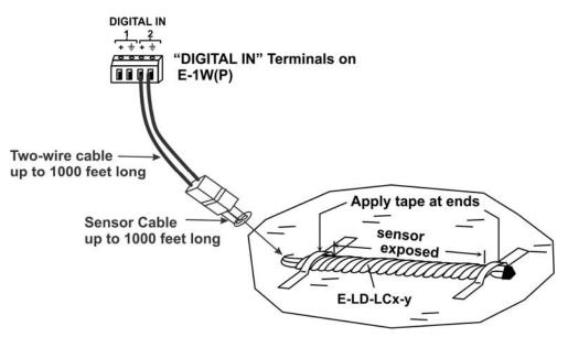
Figure 6- Secure liquid detection sensor with tape
