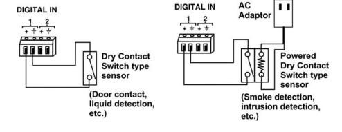
Figure 5- Terminal block for dry-contact sensors
