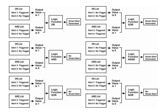
Figure 28- Examples of Smart Alert conditions
