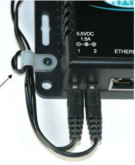
Figure 13- Use cable restraint
