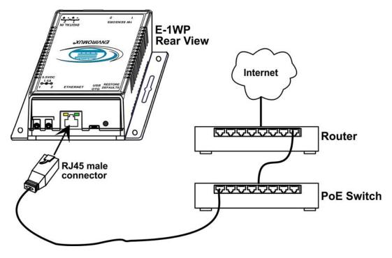
Figure 11- Connect to a PoE Switch
