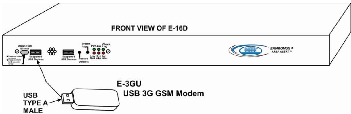
Figure 18- Install USB GSM Modem
