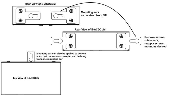
Note: The E-xD must be running firmware version 2.31 or later in order to use the E-ACDCLM with it. Refer to the E-xD manual for firmware upgrade instructions as needed. To mount multiple E-ACDCLM in close proximity to the E-16D, install an extension rail kit (NTI E-RL-16D - sold separately) and mount E-ACDCLM as seen in the illustration below.
