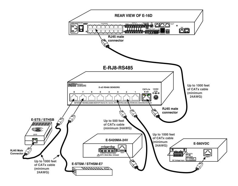
2. Connect the 12VDC power supply to the E-RJ8-RS485 and plug into power.
