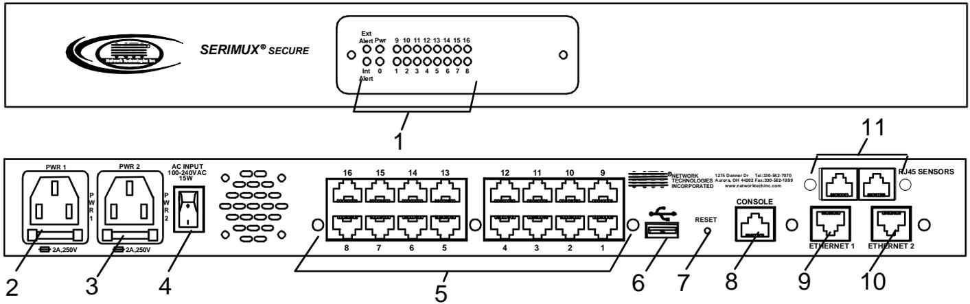
1. **STATUS LEDs**- LEDs will illuminate to indicate the SERIMUX is ON, activity on connected ports, or if there are alerts
