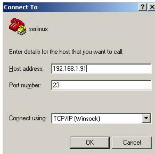
Figure 126- Telnet connection via HyperTerminal
