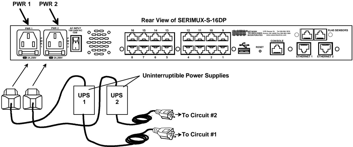
Figure 5- Power connections for SERIMUX with Dual Power option
