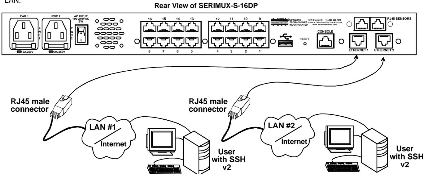
Figure 4- Connect the LAN to the SERIMUX
