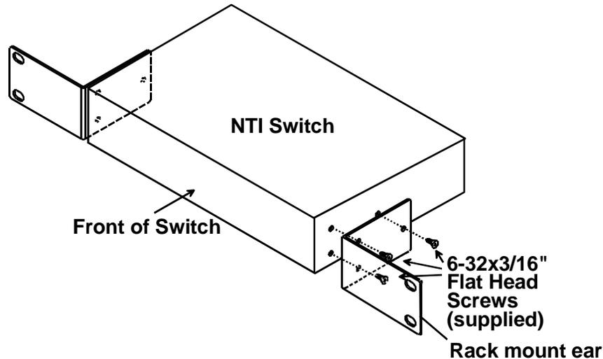
Figure 1- Secure rack mount ears to switch
