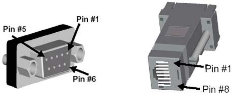
**DB-9 Female to RJ45 Pin Assignments**
