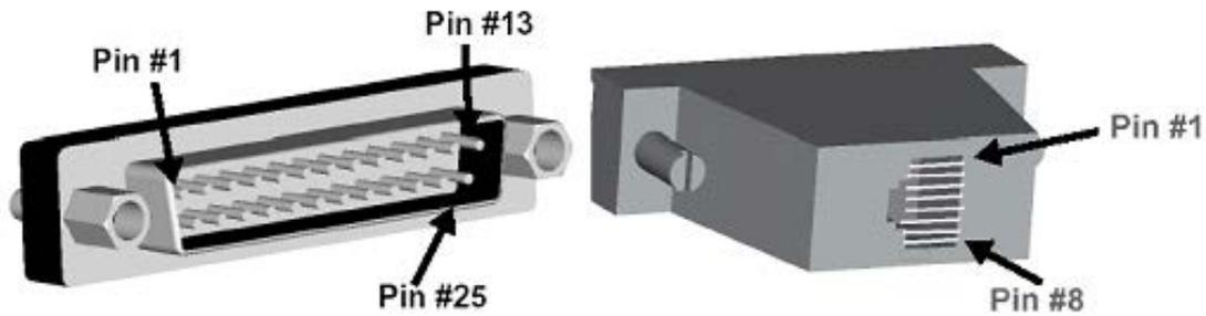
**DB-25 Male Modem to RJ45 Pin Assignment**
