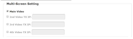
The system supports Multi-Screen feature which is useful for PC with multiple HDMI screen outputs (above):
