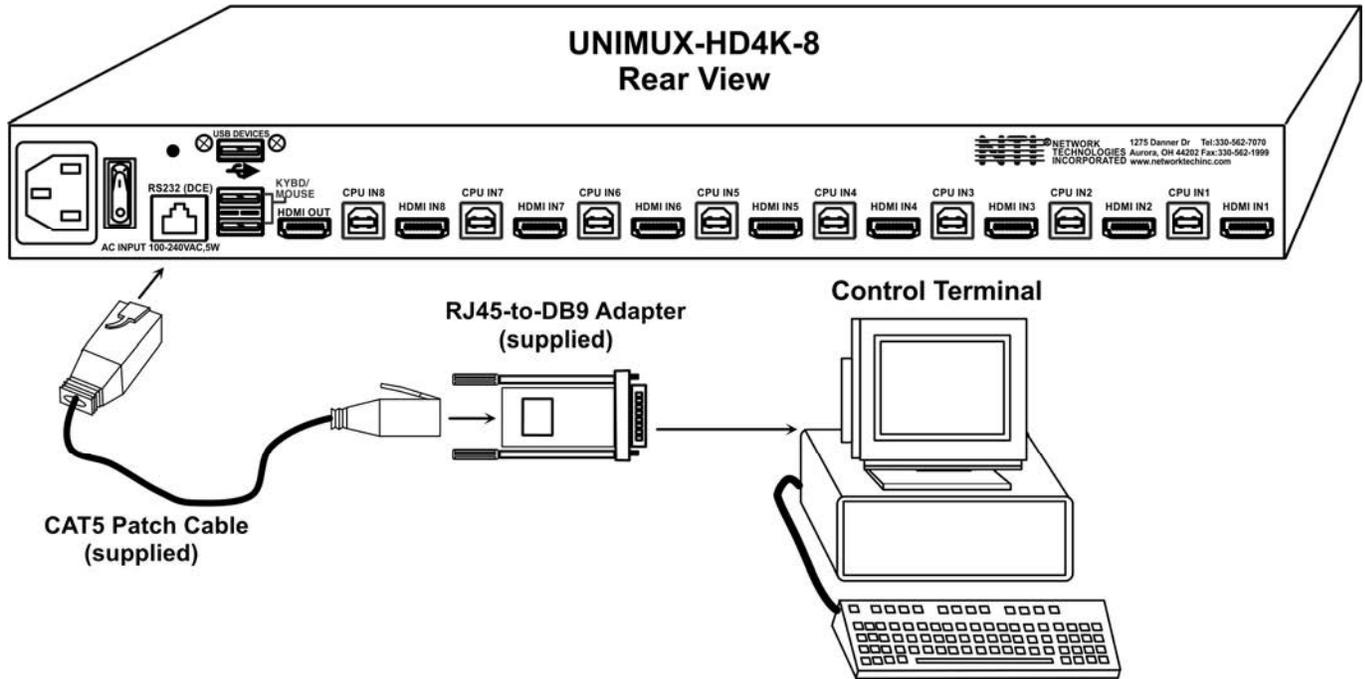
Figure 7- Connect Terminal for RS232 Control
