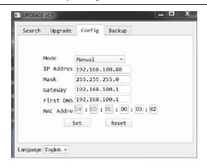
You should now be able to set your cameras IP address to one in the range of your network. You should be able to leave the subnet mask alone, unless you are configuring the camera for use across (example: 192.168.111.1) (Note that in more complex network environments you may have to request a "STATIC IP" from the IT department to prevent
