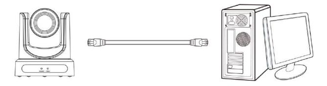
Picture 1.1 Direct connections via "cross-over" network cable
