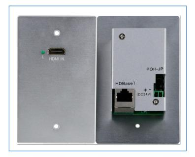
WolfPack HDBaseT-Wallplate is an HDBaseT Wallplate transmitter, it can support 1\*HDMI input, 1\*HDBaseT(RJ45) output. The resolution can up to 4k@30hz, with the POC(power over cable) function, users can only power on the HDBaseT receiver. For the transmission distance it can up to 70m at 1080P, and for 4K30Hz it can up to 35m. It's popularly used in the small meeting room, classroom or other long distance transmittion applications.
