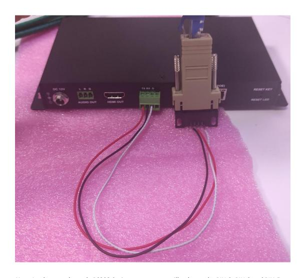
**Note 1:** when get the male RS232 9-pin connector, we will only use the PIN-2, PIN-3 and PIN-5
