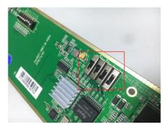
Step3: Pull all this 4-pin DIP switch to the middle position(Turn off the POC function)
