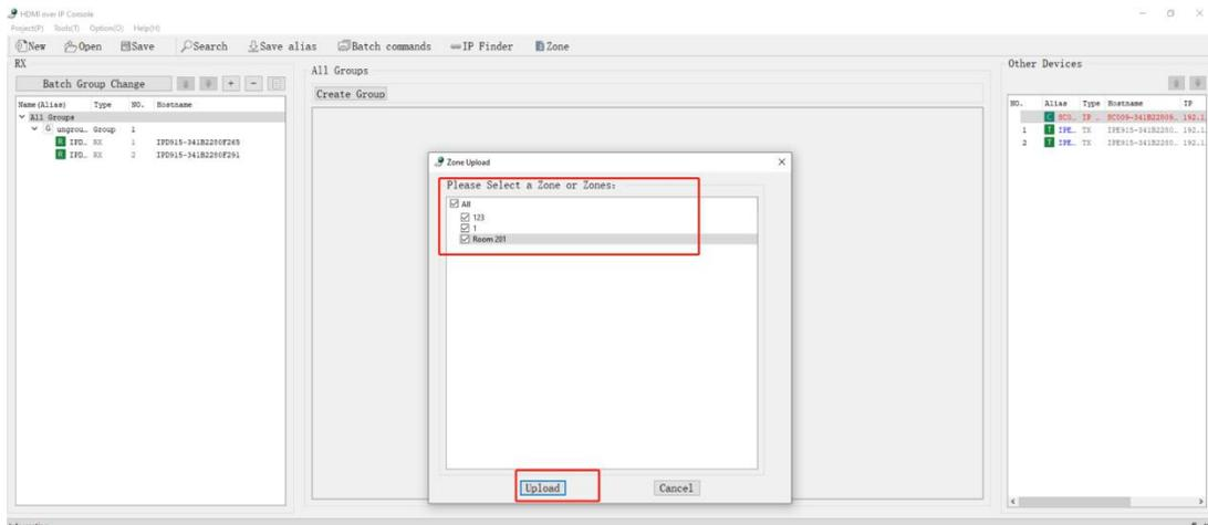
After the Zone uploaded successfully, then can use the second Windows software(VisualDMS- V1.0.9) to Login with specific Zone name for the specific control:
