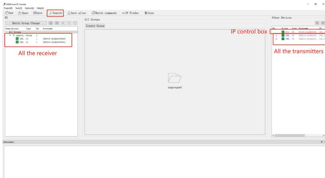
2. After find all the connected Transmitters, Receivers and the IP control box, will need to use the right click on the “IP control box” to upload the configuration:
