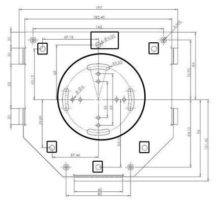
If your ceiling is made of concrete, then on the surface where the PTR robotic pan tilt head is to be installed, drill six holes spaced according to the dimensions indicated in the diagram above (enclosed by six rectangles) then use the six expansion bolts in your product package to secure the ceiling mount bracket B to the ceiling.
