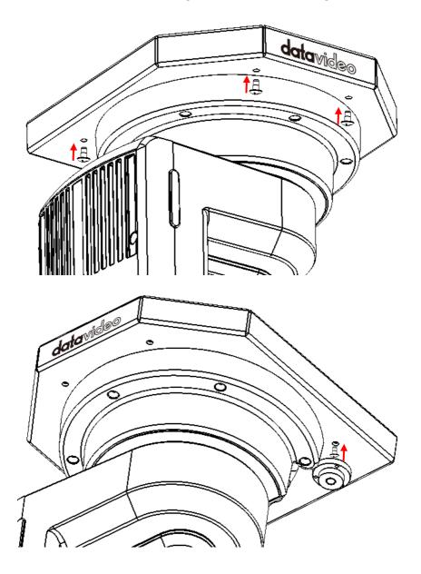
8. Finally secure your camera to the camera mount base as shown in the diagram below.
