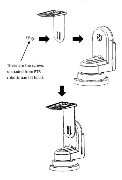
5. Secure the ceiling mount bracket A to the base of the PTR robotic pan tilt head.
