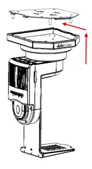
7. Insert the four M4 x 8mm screws (black) into each of the four holes in the four corners of the ceiling mount bracket A then tighten.
