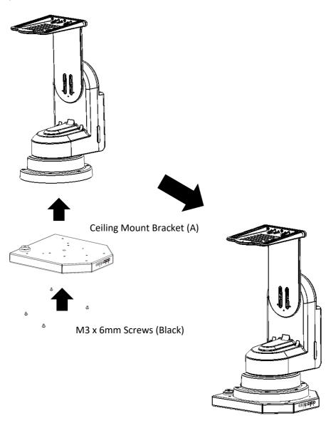
6. As shown in the diagram, push the ceiling mount bracket A along with the PTR robotic pan tilt head into the ceiling mount bracket B secured to the ceiling then backwards until the two brackets click into place.
