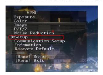
8. Please press the "down-arrow" button from the PTC-280NDI remote controller to move to the "USB UPGRADE" option in the "Setup" page.
