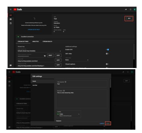
5. Users can see the Stream Key and Stream URL that are provided by the Youtube streaming platform. Please copy the stream key and stream URL and then paste them into the "First Stream MRL" within the "Network" option of the PTC-280NDI Web UI according to the following format (Stream URL/Stream Key). Please click "On" and please check the checkboxes of "Audio" and "Video".
