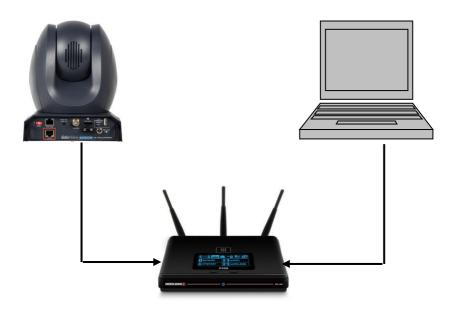
In order to enable the DHCP mode of the camera, please select "Dynamic IP Address" from the "IP Configuration Type" drop-down menu for assigning a dynamic IP address to PTC-280NDI by the router. After that, please click the "Apply" button to save the new settings and then please reboot the PTC-280NDI.
