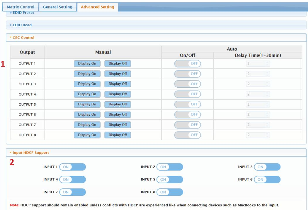
1. CEC Control: Turn on/off a display connected to the HDMI output. Turn on/off the auto function and adjust the delay time.
