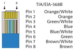
The TCP/IP port requires a standard straight-through Category 5 or greater cable with the TIA/EIA-568B crimp pattern for optimal operation.
