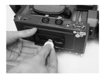
Secure the quick release camera plate to the tripod head with DAC-07 and Camera attached.
