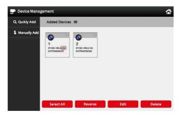
Note: In the PJZ control page, you can enter the last digits of the camera's IP address directly on the keyboard and then press the [Address] button to connect the PTZ camera In this example, you may enter "239" to add the camera at 192 168 0 239; please use the actual last digits of your camera's specific IP address
