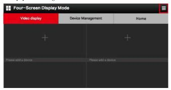
Click the pop-up menu bars at the upper right corner of the PTZ mode screen, then select [Device Management] to enter the device management interface as shown below
