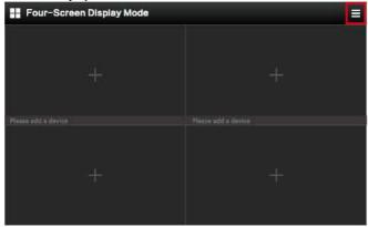
In [PTZ Mode], click the at the upper right corner Select [Video Display] to display a four-image window Click on the screen to open the [Device Add] dialog box Double-click the IP address of the camera to display the screen
