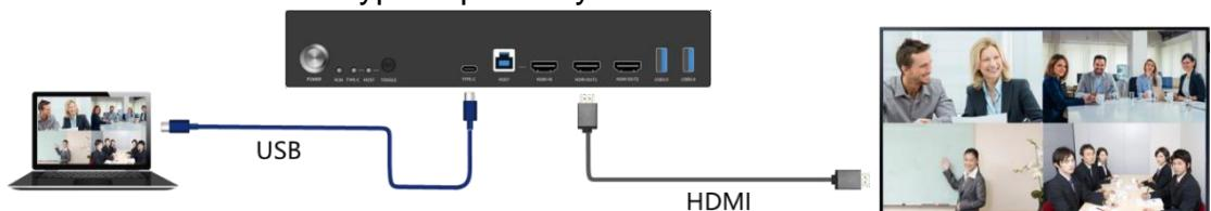
2. Use USB Type-B port and HDMI IN port for connection.
