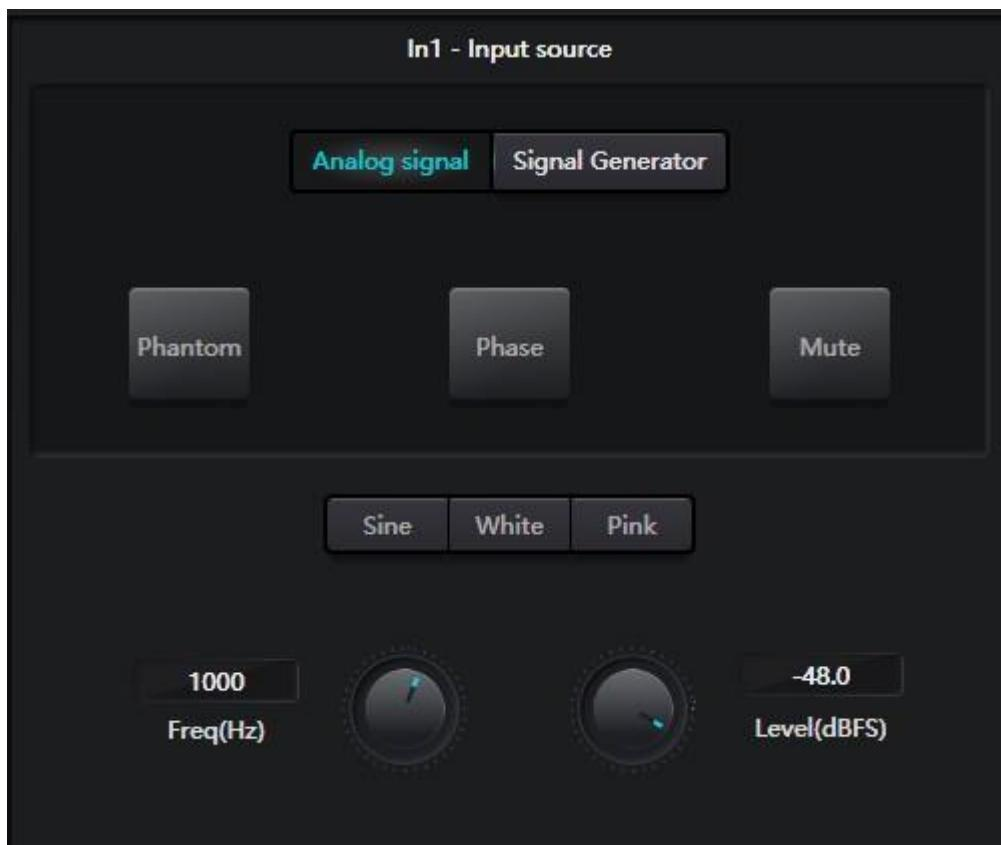
**Phantom power supply:** Feed the external capacitive microphone, enabled when connected to the microphone. Do not open without power supply, in case of damage to external equipment.
